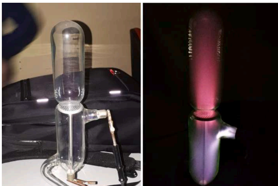
Fig. 3. A Canal rays tube. Notice the perforated cathode in the middle of the tube.
